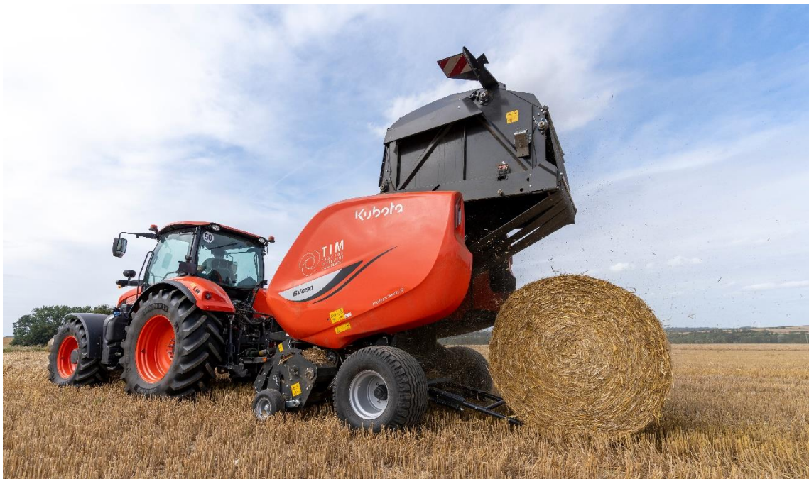
Picture: Kubota BV6190 designed for high-quality bales up to 1.85m
