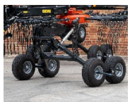
Kubota RA2071T Evo - Tandem wheels
