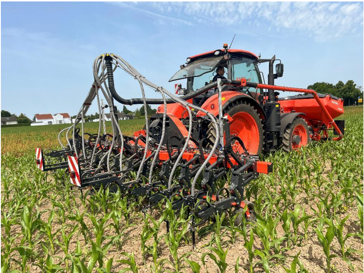
Fertiliser application whilst weeding with the Kubota IC3000F, front hopper SH1600 and distribution head
